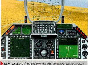
**NEW PANELING** IF-16 simulates the MLU instrument package, which includes color multi-function displays.
